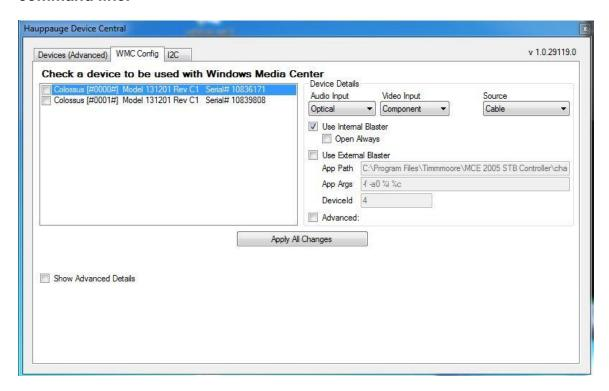
Under app path enter the path and executable you will be passing the command line too. Arguments allows you to pass information such as channel number or device id %c will do channel number %i will do device id. Please note we do not provide support for external blasters.
