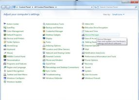
c) If the HDPVR driver is not currently installed the HDPVR or Colossus will appear under the "Other devices" category. If an HDPVR driver is installed the HDPVR will appear under the "Sound, video and game controllers" category. If the device does not appear in either location please check your connections.
