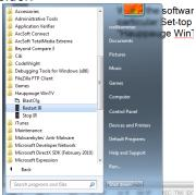
a) The BlastCfg window will open. Configure for your particular STB and test by clicking on the "Send" button. The <u>STB should tune to the indicated channel</u> (123 by default).
